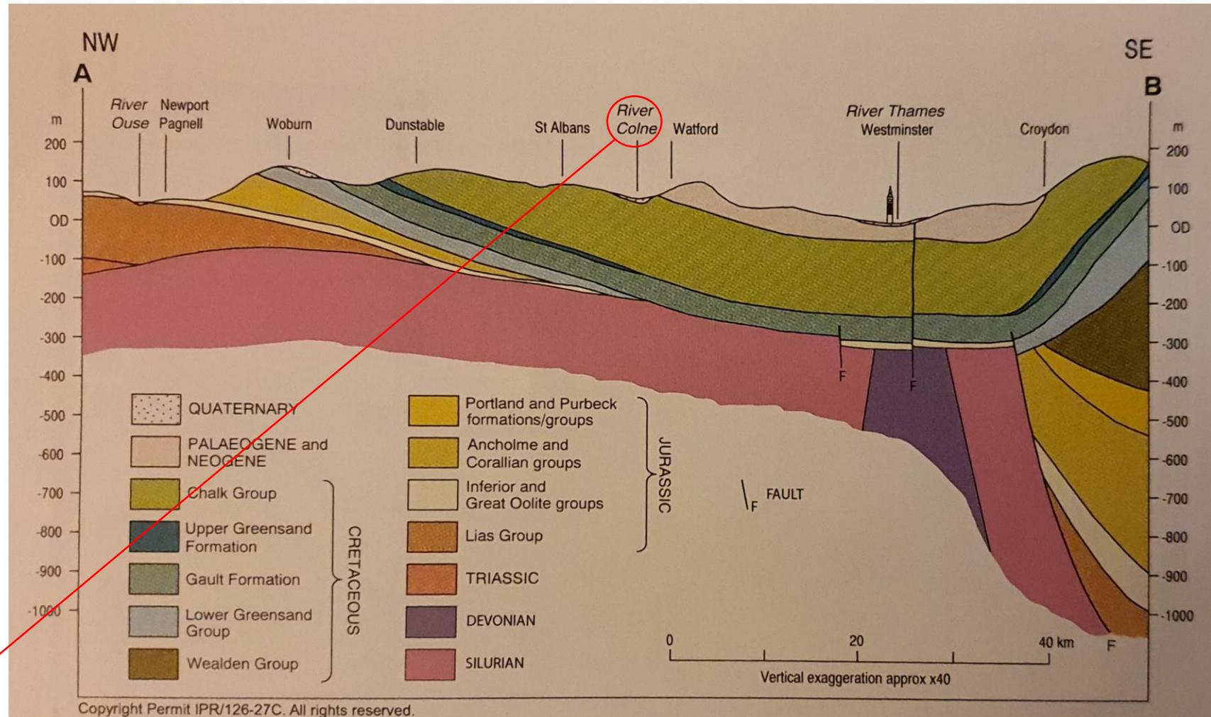
**Figure 4.** Cross-section of the London Basin showing how the older outcrops can be seen on either side of the Thames Valley. The syncline is superimposed on the older anticline of Palaeozoic rocks. IPR/126-27C British Geological Survey © NERC. All rights reserved.
