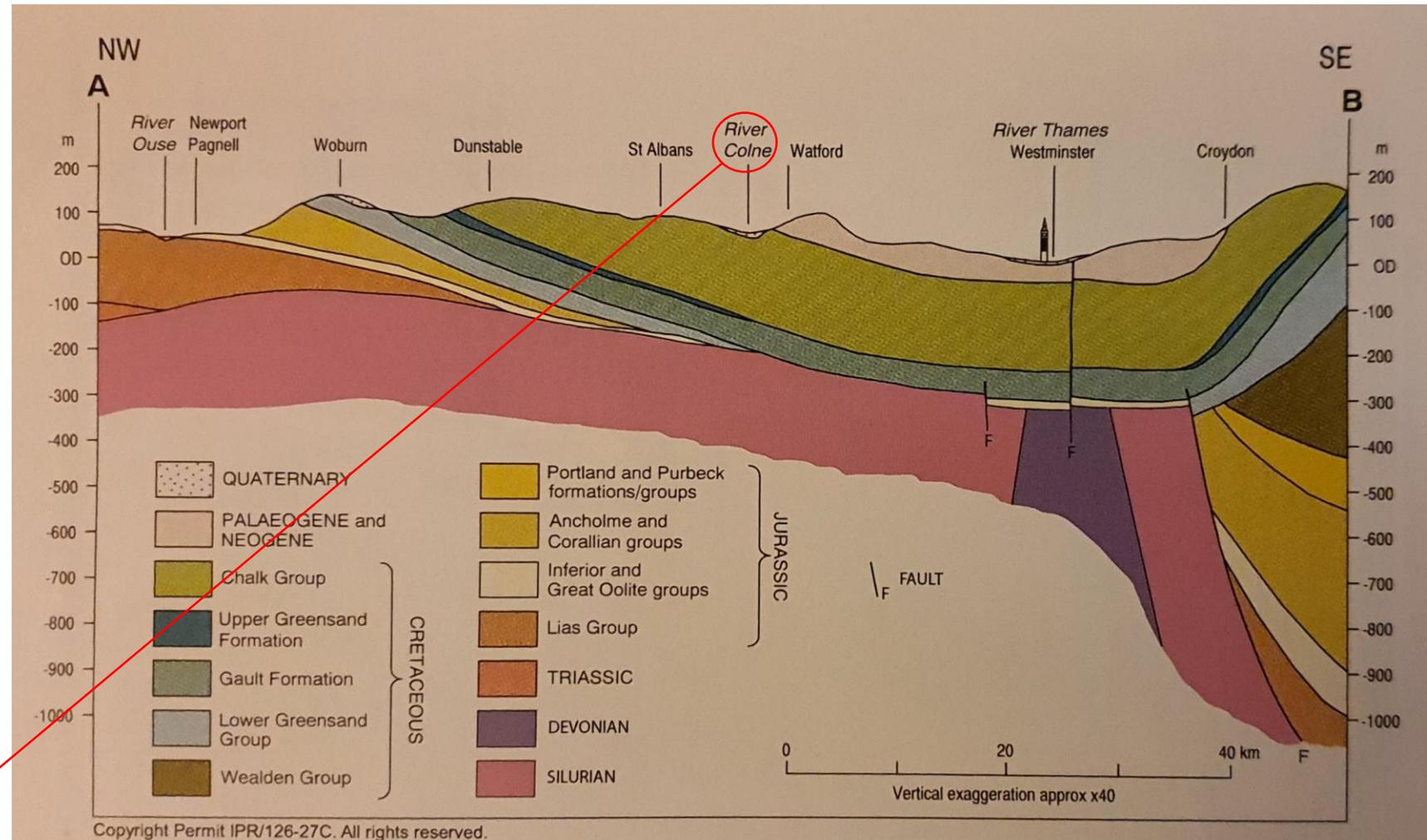
**Figure 4.** Cross-section of the London Basin showing how the older outcrops can be seen on either side of the Thames Valley. The syncline is superimposed on the older anticline of Palaeozoic rocks. IPR/126-27C British Geological Survey © NERC. All rights reserved.
