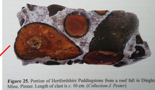
Figure 25. Portion of Hertfordshire Puddingstone from a roof fall in Dingles Mine, Pinner. Length of clast is c. 10 cm. (Collection J. Pester)
