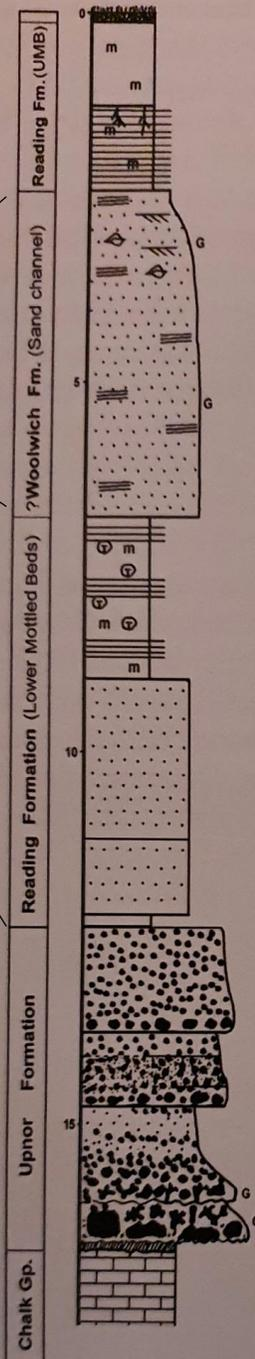
**Figure 24.** Detailed log of rock overlying Dingles Chalk Mine, Pinner, drawn by Jackie Skipper from exposures due to roof collapse and core obtained by Mark Bradley. UMB = Upper Mottled Beds, G = glauconite (*amended from Gallois, 1998 and reproduced with kind permission of HHGS*).
