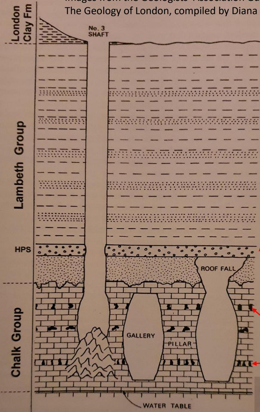
Figure 22. Section through the Dingles Mine showing the geology and method of working. HPS = Hertfordshire Puddingstone. (After Gallois, 1982)
