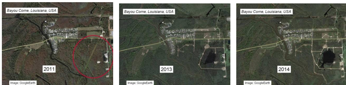
Development of subsidence above brine extraction, Bayou Corne, Louisiana
